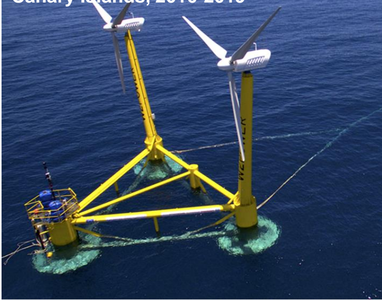
6th Scale FOWT Demonstrator, PLOCAN, Canary Islands, 2016-2019
